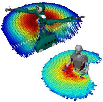
Visualization of reachability and manipulability for the ARMAR-6 and ARMAR-III robots
