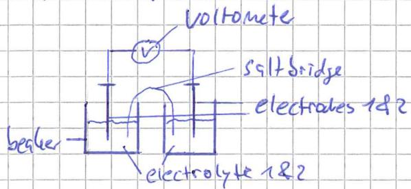
The salt bridge consists of a cut filter paper soaked in the corresponding salt solution.
