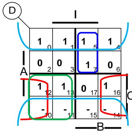
$$D = \bar{A} + C \bar{B} + C \bar{I} + \bar{C} B I$$
