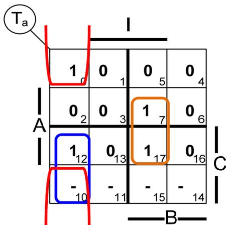
$$T_a = \bar{I} \bar{B} \bar{A} + C \bar{B} \bar{I} + IBA$$
