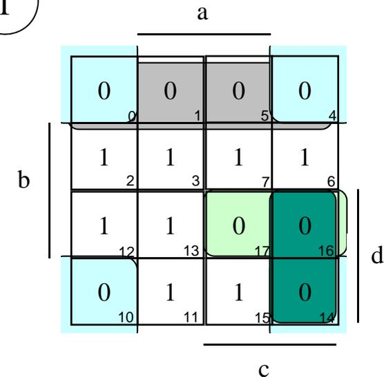
The Karnaugh map for function f is a 4x4 grid with cells numbered 0 to 15. The variables are a (horizontal), b (vertical), c (horizontal), and d (vertical). The cells contain the following values:
