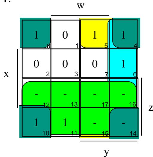
$$f = z + \overline{w}y + \overline{x}\overline{w} + y\overline{x}$$
