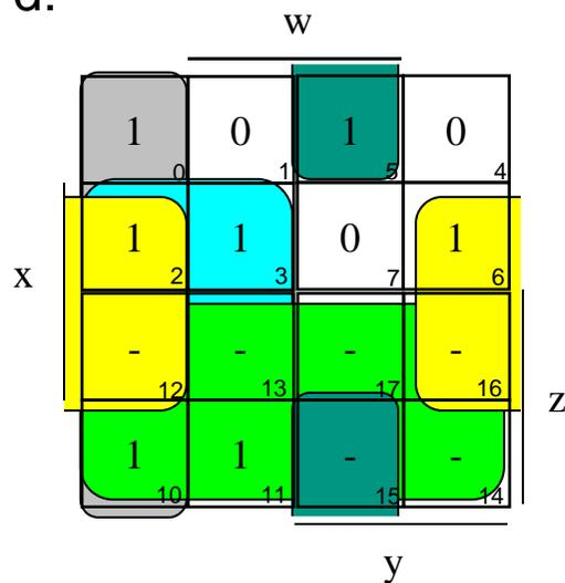
$$d = z + \overline{w}y + x\overline{w} + x\overline{y} + wy\overline{x}$$
