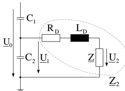
$$\text{mit } \underline{Z}_2 = R_D + \ddot{u}^2 R_B + j\omega L_D$$
