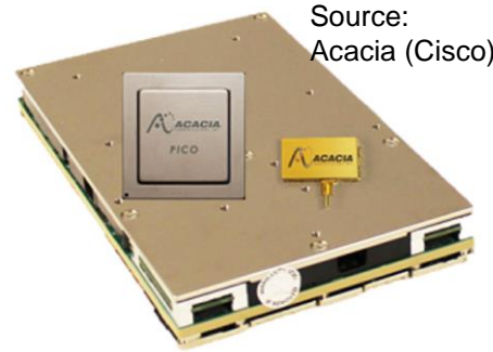
1.2 Tb/s Coherent Optical DSP ASIC
