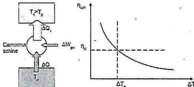
$$\eta_{WP} = \frac{E_{\text{Nutz}}}{E_{\text{Aufwand}}} = \frac{|Q_1|}{\Delta W_{\text{ges}}} = \frac{|Q_1|}{|Q_1| - Q_2} = \frac{1}{\eta_{\text{Carnot}}} = \frac{T_1}{T_1 - T_2} = \frac{T_1}{\Delta T} > 1$$
