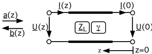
$$\underline{U}(z) = \underline{U}_H(0)e^{\gamma z} + \underline{U}_R(0)e^{-\gamma z} = \sqrt{Z_L}(\underline{a}(z) + \underline{b}(z))$$
