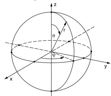
Azimuth:  $\psi$       Elevation:  $\theta$
