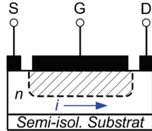
Metal-Semiconductor Field Effekt Transistor (**MESFET**) :
