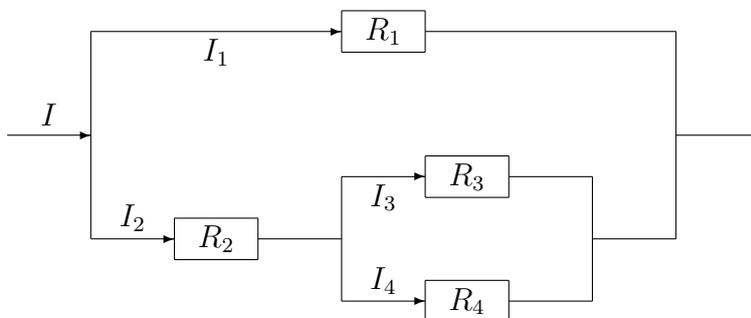
Es gelte  $I = 1 [A]$  und  $R_1 = R_2 = R_3 = \alpha [\Omega]$  sowie  $R_4 = \beta [\Omega]$ .
