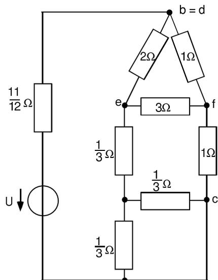
$$R_d = \frac{2\Omega \cdot 1\Omega}{2\Omega + 3\Omega + 1\Omega} = \frac{2}{6}\Omega = \frac{1}{3}\Omega$$
