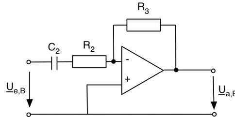
$$R_1 = 10k\Omega, R_2 = 1k\Omega, R_3 = 10k\Omega, C_1 = C_2 = 20nF.$$
