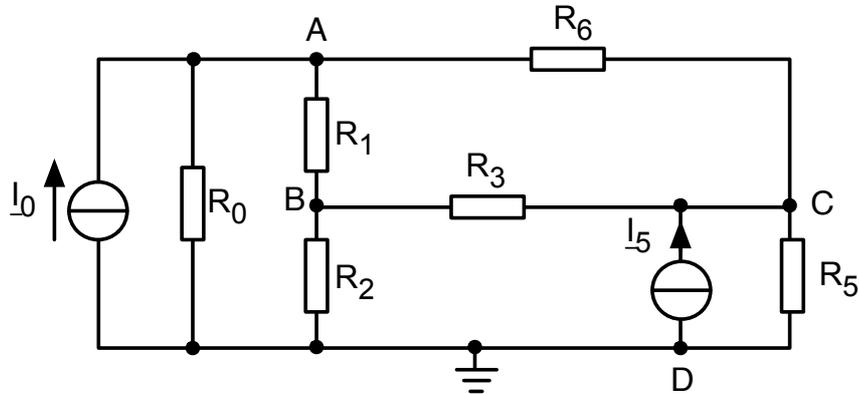
$$\begin{bmatrix} \left( \frac{1}{R_0} + \frac{1}{R_1} + \frac{1}{R_6} \right) & -\frac{1}{R_1} & -\frac{1}{R_6} \\ -\frac{1}{R_1} & \left( \frac{1}{R_1} + \frac{1}{R_2} + \frac{1}{R_3} \right) & -\frac{1}{R_3} \\ -\frac{1}{R_6} & -\frac{1}{R_3} & \left( \frac{1}{R_3} + \frac{1}{R_5} + \frac{1}{R_6} \right) \end{bmatrix} \begin{pmatrix} U_A \\ U_B \\ U_C \end{pmatrix} = \begin{pmatrix} I_0 \\ 0 \\ I_5 \end{pmatrix}$$
