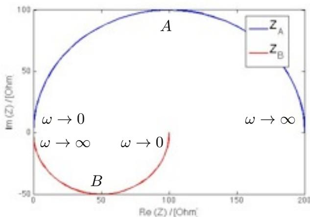
$$\text{c) } \underline{Y}_B(\omega) = \frac{1}{R} + j\omega C$$
