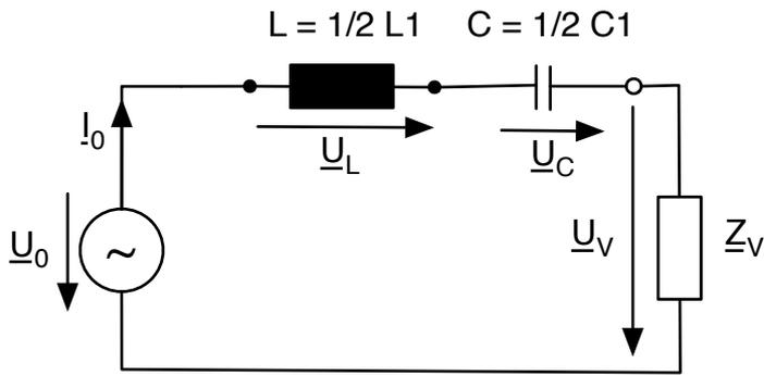
$$\underline{U}_L = j\omega L I_0 = j\omega \frac{1}{2} L1 I_0 = j \frac{2\pi}{2\pi} \text{kHz mH A} = j1 \text{ V}$$
