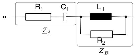
$$\underline{Z}_A = R_1 - \frac{j}{\omega C_1}$$
