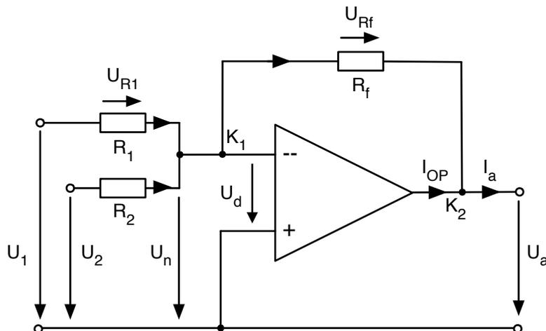
$$K_1: (U_1 - U_n) \frac{1}{R_1} + (U_2 - U_n) \frac{1}{R_2} - (U_n - U_a) \frac{1}{R_f} = 0$$
