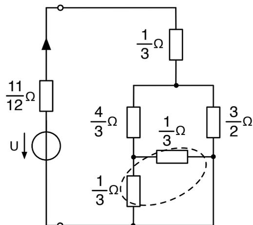
$$\frac{1}{3}\Omega \parallel \frac{1}{3}\Omega = \frac{\frac{1}{3} \cdot \frac{1}{3}}{\frac{1}{3} + \frac{1}{3}}\Omega = \frac{1}{6}\Omega$$
