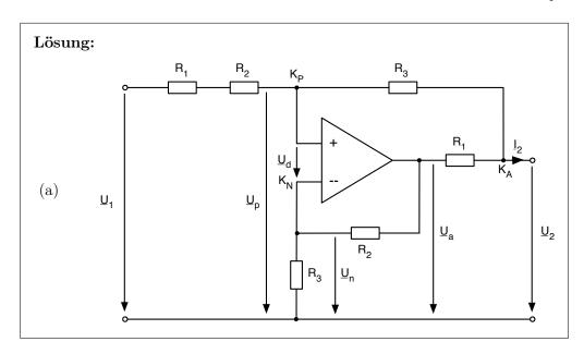
$$K_P: \frac{\underline{U}_1 - \underline{U}_p}{R_1 + R_2} + \frac{\underline{U}_2 - \underline{U}_p}{R_3} = 0$$
