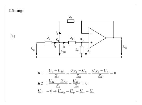
$$K_{2}: \frac{\underline{U}_{K_{1}} - \underline{U}_{a}}{\underline{Z}_{2}} - \frac{\underline{U}_{a}}{\underline{Z}_{4}} = 0$$
