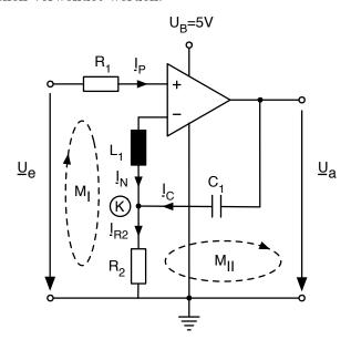
$$\begin{array}{rcl} M_I:\underline{U}_e & = & R_1\underline{I}_P + \underline{Z}_L\underline{I}_N + R_2\underline{I}_{R_2} \\ \\ M_{II}:\underline{U}_a & = & R_2\underline{I}_{R_2} + \underline{Z}_C\underline{I}_C = R_2\underline{I}_{R_2} + \underline{Z}_C\underline{I}_{R_2} = (R_2 + \underline{Z}_C)\underline{I}_{R_2} \end{array}$$
