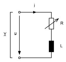
$$\begin{array}{rcl} \omega_0 L & = & 10 \, \Omega \\ & \underline{\hat{U}} & = & 10 \, V \cdot e^{j\pi} \\ & R & \in & [0 \dots \infty) \, \Omega \end{array}$$
