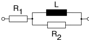
$$\underline{Z} = R_1 + \frac{R_2 \cdot j\omega L}{R_2 + j\omega L}$$
