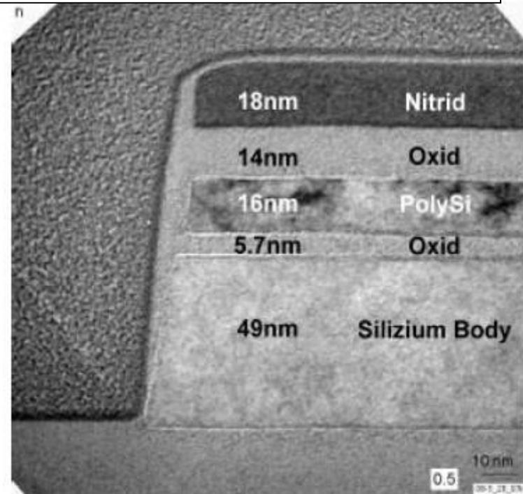
Fig. 9: TEM picture of a floating gate memory cell: Cross section of the Silicon channel with a 5.7nm thick  $\text{SiO}_2$  tunnel oxide and a 16nm poly Si floating gate. On top is a Nitride dielectric serving as a hard mask for etching the floating gate and Si-body.
