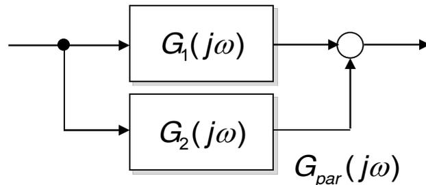
$$G_{par}(j\omega) = G_1(j\omega) + G_2(j\omega)$$
