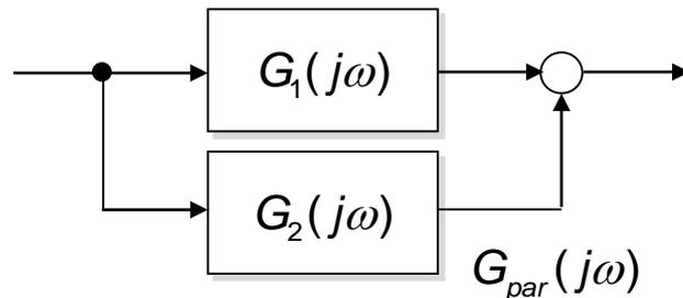
$$G_{par}(j\omega) = G_1(j\omega) + G_2(j\omega)$$
