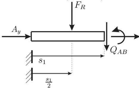
$$\begin{aligned} F_R &= q_0 s_1 \\ \Rightarrow Q_{AB} + F_R &= 0 \\ Q_{AB} &= -q_0 s_1 \end{aligned}$$
