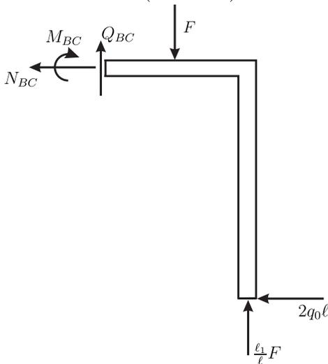
$$\begin{aligned} N_{BC} + 2q_0 l &= 0 \\ N_{BC} &= -2q_0 l \end{aligned}$$
