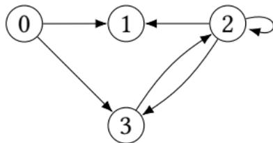
$$\begin{array}{c} \begin{array}{cccc} & 0 & 1 & 2 & 3 \\ \begin{array}{c} 0 \\ 1 \\ 2 \\ 3 \end{array} & \begin{pmatrix} 0 & 1 & 0 & 1 \\ 0 & 0 & 0 & 0 \\ 0 & 1 & 1 & 1 \\ 0 & 0 & 1 & 0 \end{pmatrix} \end{array} \end{array}$$
