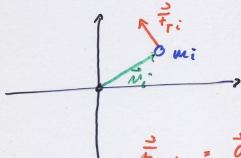
$$\begin{aligned}\vec{f}_{r_i} &= \vec{a}_I \cdot m_i \\ \Rightarrow a_r &= \frac{\vec{f}_{r_i}}{m_i} = \alpha \cdot r_i\end{aligned}$$
