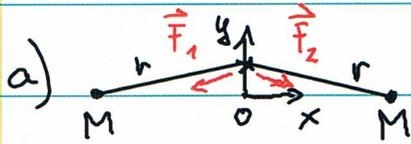
$$\begin{aligned} \vec{F} &= \vec{F}_1 + \vec{F}_2 = G \frac{mM}{r^2} \frac{1}{r} \begin{pmatrix} -x \\ -y \end{pmatrix} + G \frac{mM}{r^2} \frac{1}{r} \begin{pmatrix} x \\ -y \end{pmatrix} \\ &= G \frac{mM}{r^3} \begin{pmatrix} 0 \\ -2y \end{pmatrix} = G \frac{mM}{(x^2+y^2)^{3/2}} \begin{pmatrix} 0 \\ -2y \end{pmatrix} \end{aligned}$$
