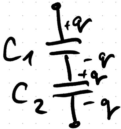
$$\frac{1}{C} = \frac{1}{C_1} + \frac{1}{C_2}, \quad \frac{1}{C} = \sum_i \frac{1}{C_i}$$
