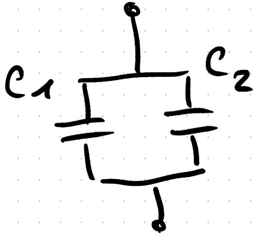
$$C = C_1 + C_2 ; \quad C = \sum_i C_i$$
