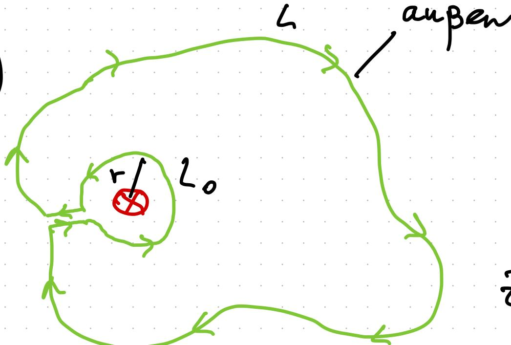
$$\oint_L \vec{B} d\vec{\ell} = \underbrace{\oint_L \vec{B} d\vec{\ell}}_{L_0} + \underbrace{\oint_{L_0} \vec{B} d\vec{\ell}}_{L_0 S} + \underbrace{\oint_{L_0 S} \vec{B} d\vec{\ell}}_{L_0 Q} = 0 \text{ (außen)}$$
