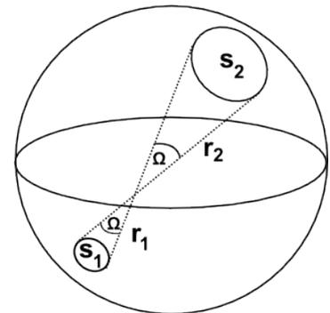
$$\begin{aligned} \frac{\Omega}{4\pi} &= \frac{s}{4\pi r^2} & \rightarrow s &= \Omega r^2 \\ & & \rightarrow s_1 &= \Omega r_1^2 \\ & & \rightarrow s_2 &= \Omega r_2^2 \end{aligned}$$
