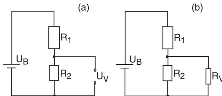
Zahlenwerte:  $R = R_1 + R_2 = 1 \text{ k}\Omega$ ,  $U_B = 9 \text{ V}$ ,  $U_V = 3 \text{ V}$
