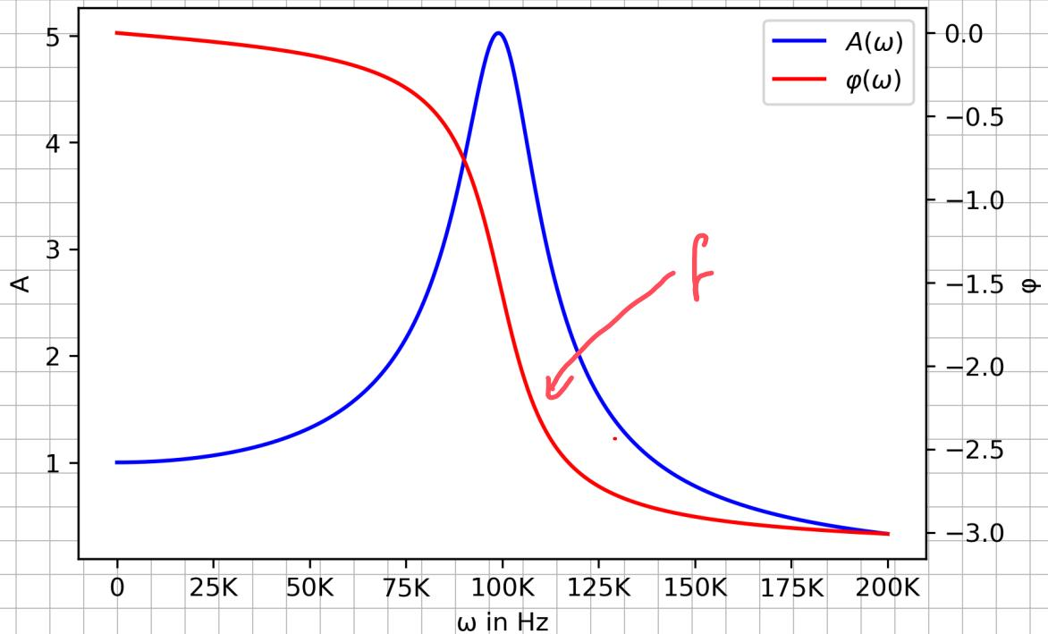
b)  $|U_a(t)| = \left| \frac{\tilde{U}_e(t)}{i\omega RC - \omega^2 LC + j} \right| = \left| \frac{U_0 e^{j\omega t}}{i\omega RC - \omega^2 LC + j} \right| = U_0 A(\omega) \cos(\omega t + \varphi(\omega))$  ✓
