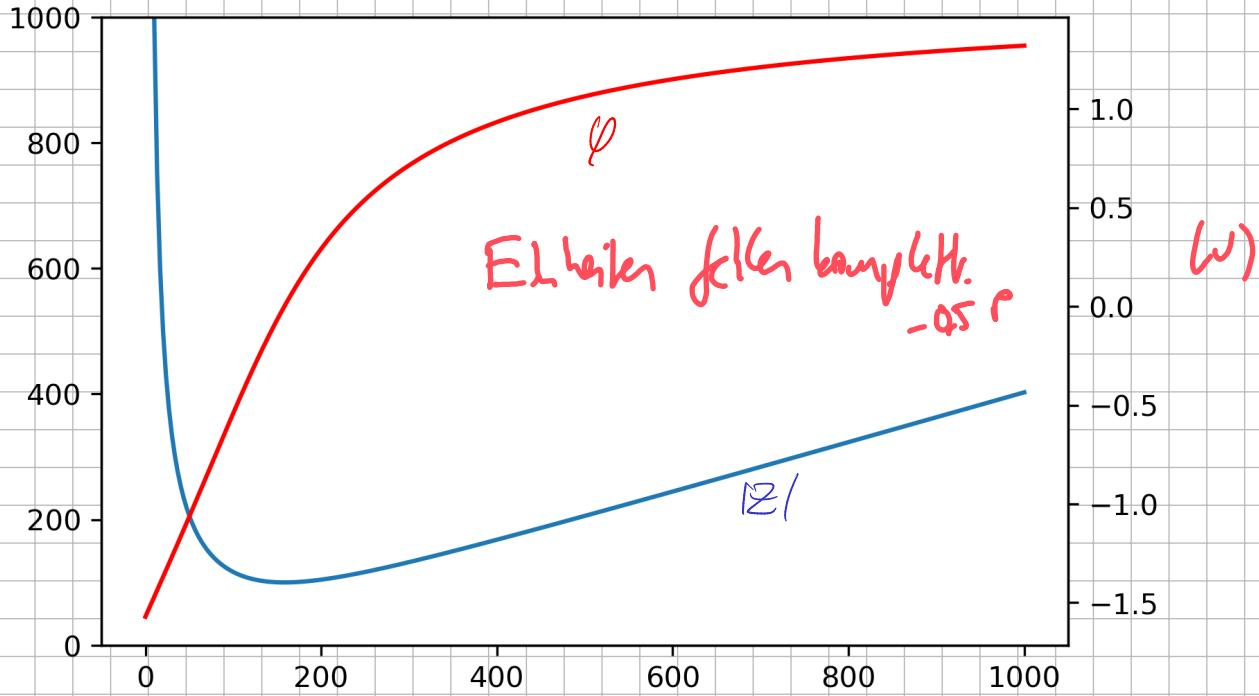
$$\langle P \rangle = \frac{U_e H}{|Z|} \cos(\varphi) = \frac{U_0^2}{2|Z|} \cos(\varphi) = 140,657 \text{ W} \quad f \quad \checkmark$$
