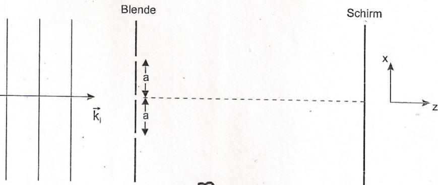
$$\frac{1}{I_0} \sim \left| \int_{-\infty}^{\infty} T(x) e^{ik_x x} dx \right|^2 = \left| \int_{-\infty}^{\infty} (\delta(x) + \delta(x-a) + \delta(a+x)) e^{ik_x x} dx \right|^2$$
