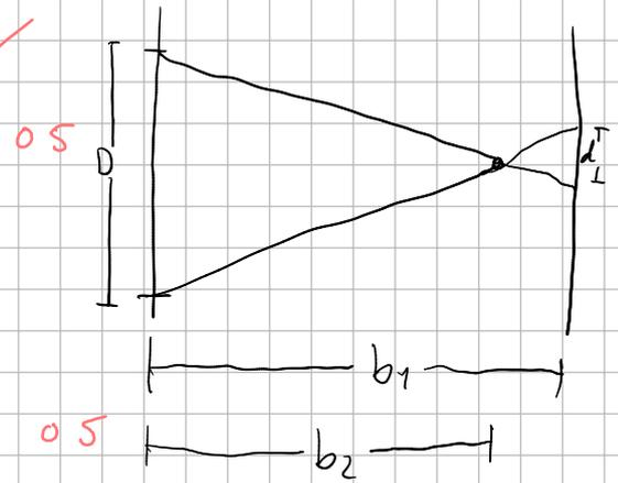
c) Für  $g_2 = 7 \text{ m}$   $d \stackrel{!}{=} 50 \mu\text{m}$   $D = \frac{d \cdot b_2}{|b_2 - b_1|}$
