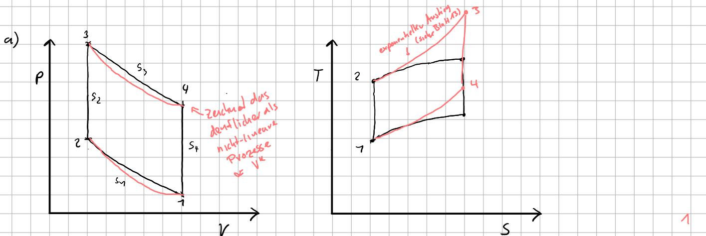
b) Schritt 1:  $pV^k = \text{const}$        $pV = TnR \Rightarrow p_1 = \frac{T_1}{V_b} nR$        $f = \frac{2}{k-1}$
