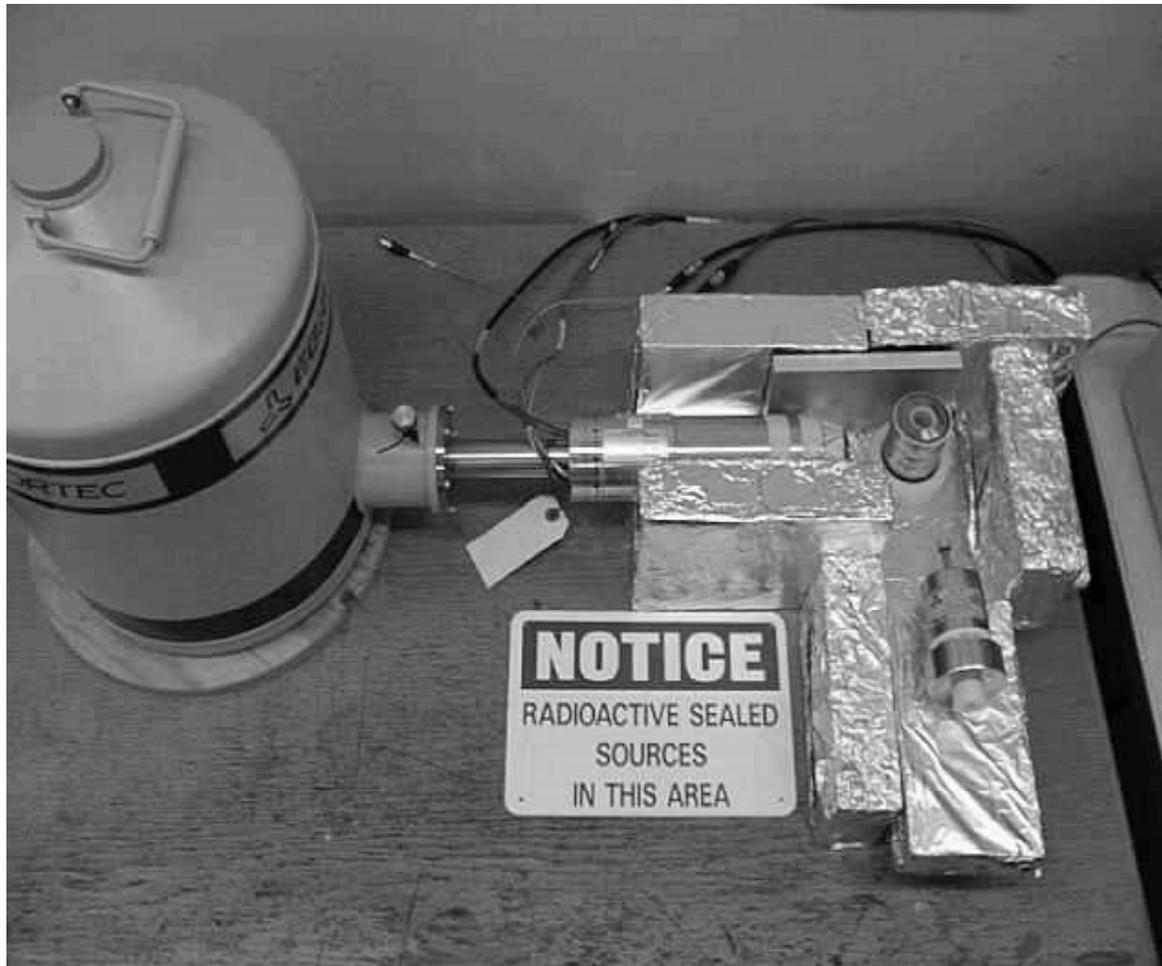
A picture of the experimental setup. The  $^{241}\text{Am}$  source is the small disk at the end of the rod coming out of the cylinder in the bottom right-hand corner of the picture.
