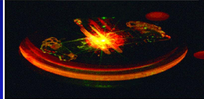
**LAB ON A CHIP COMES CLOSER - A biocavity laser - a VCSEL capped by a glass plate enclosing a blood sample, all about the size of a quarter - is excited by a pump laser in Paul Gourley's lab. The VCSEL device can produce information about the state of millions of blood cells in a few minutes. Download 150dpi jpg image, 'VCSEL.jpg', 1.5MB**
