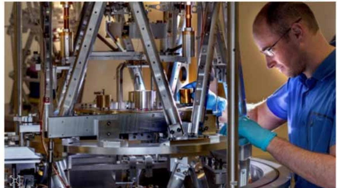
All change: work on the redefinition of the kilogram was carried out using a Kibble balance. (Courtesy: BIPM)
