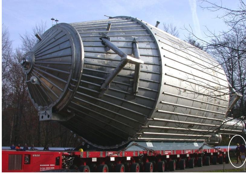
Figure 2: Current application example of a MAC-E filter: the main spectrometer of the KATRIN experiment.
