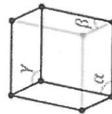
rhombohedral: all side lengths equal. all angles equal, but not right angles.
