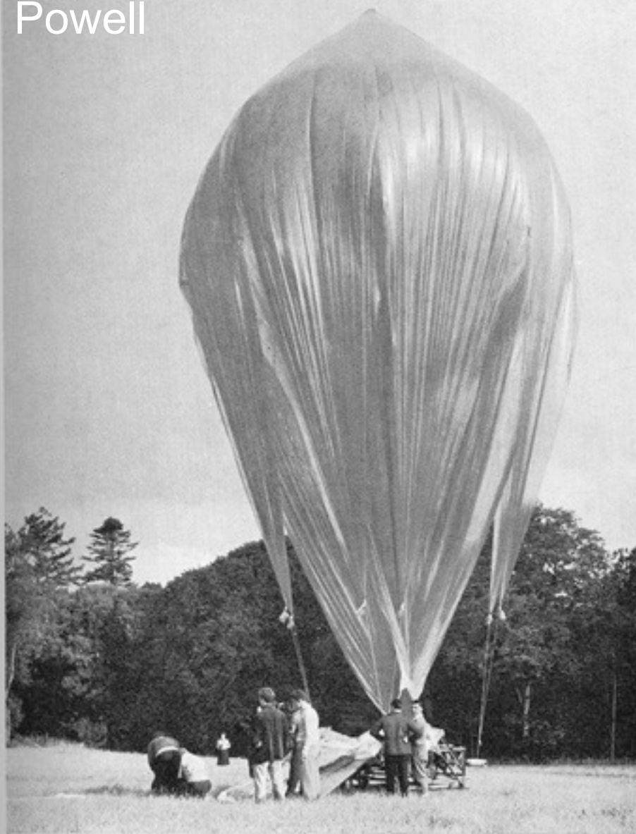
Fig. 1. Inflation of balloon of polyethylene just after dawn. The balloon has a total length of about 120 ft. and most of the fabric is on the ground. Such a balloon can in favourable conditions give level flight at about 90,000 ft. for many hours with a load of 40 kg.
