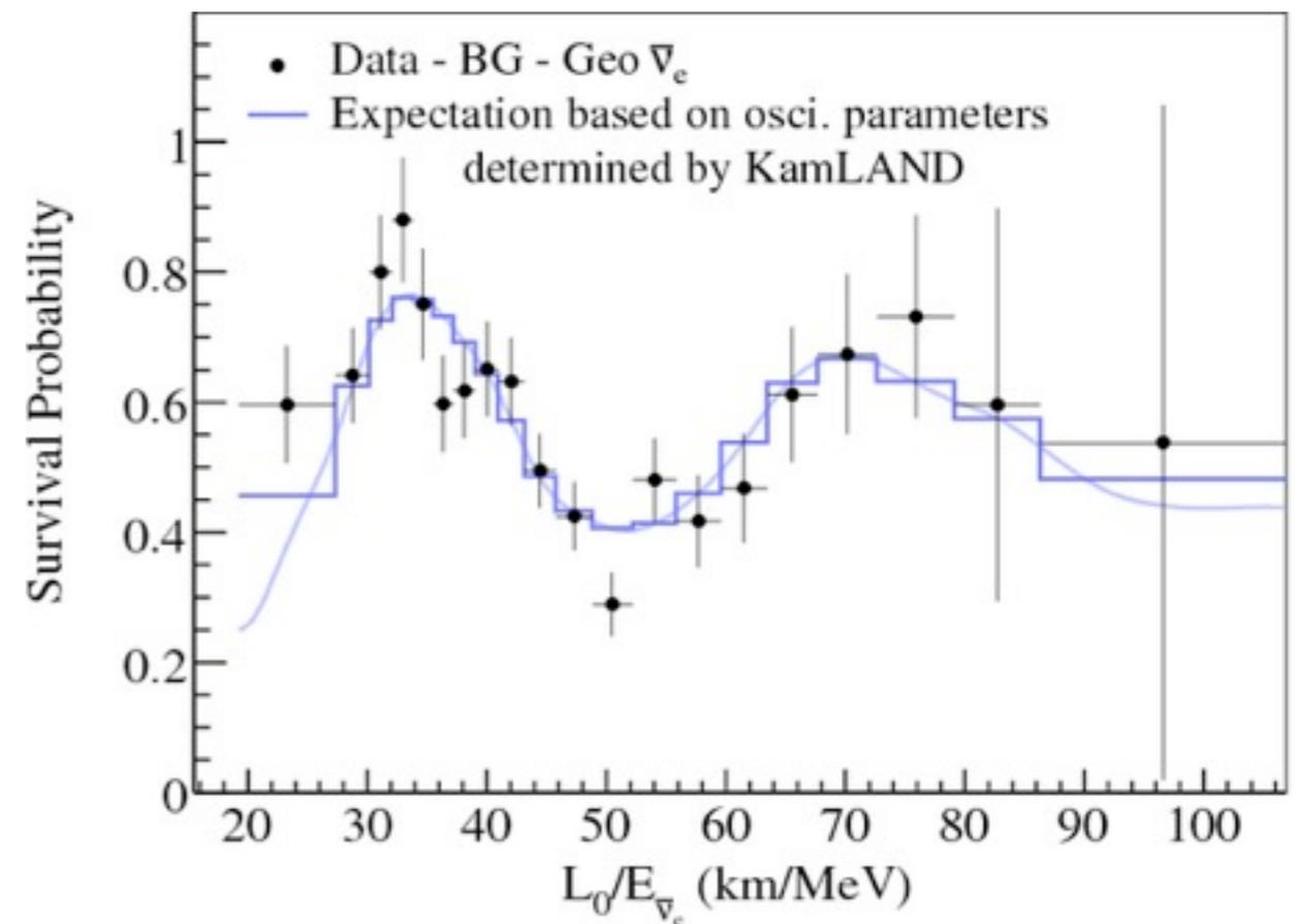
Ratio of the background and geo-neutrino subtracted anti-neutrino spectrum to the expectation for no-oscillation as a function of  $L/E$ .  $L$  is the effective baseline taken as a flux-weighted average ( $L=180\text{km}$ ). The histogram and curve show the expectation accounting for the distances to the individual reactors, time-dependent flux variations and efficiencies. The figure shows the behavior expected from neutrino oscillation, where the electron anti-neutrino survival probability is:
