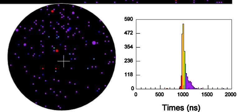
Figure 2. Examples of (a) electron neutrino and (b) muon neutrino events observed in Super-Kamiokande. The sizes of the circles in this figure show the observed light intensity. Also, the color of the circles shows the timing information of the observed light.
