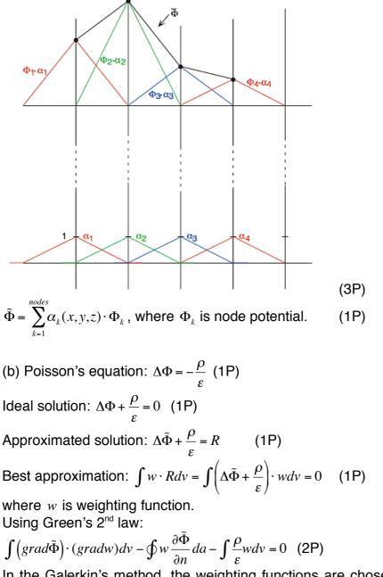
In the Galerkin's method, the weighting functions are chosen to be the basis functions:  $w_l(x,y,z) = \alpha_l(x,y,z)$ . (1P)
