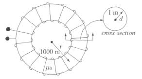
(Hint: the magnetic field strength in the torus can be considered constant along the radial direction approximately, since r >> d.)
