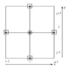
The computing molecule delivers one linear equation for each node => A linear equation system Ax = g has to be solved for the whole system. Matrix A has size n\*n for n nodes;
