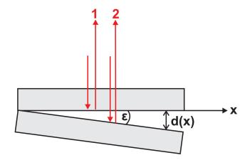
Parallel light ( $\lambda = 500 \, \mathrm{nm}$ ) under normal incidence leads to 10 interference stripes per cm due to the interference between ray 1 and 2 denoted in the figure (assume that  $\epsilon$  is so small that ray 2 exits parallel to the incident light).
