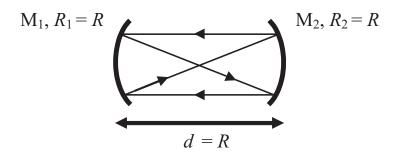
Using matrix optics, show that a ray moving under an arbitrary angle to the optical axis from the left mirror to the right reaches its intial state after four reflections. This means that the ray does not leave the resonator.
