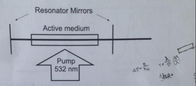
A solid state laser is realized by putting a Ti<sup>3+</sup>-doped sapphire (Ti;Sa) crystal as gain material into a Fabry-Pérot cavity of length d=30 cm and a Finesse(F) You may neglect the refractive index of the crystal for your calculations.
