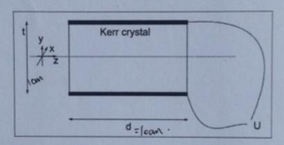
and impinges on a single Kerr cell. A transverse electrical field  $E_y$  is applied to this Kerr crystal of thickness  $t=1\,\mathrm{cm}$  and length  $d=10\,\mathrm{cm}$ . For a voltage  $U_1=100\,\mathrm{V}$  you observe an additional phase shift of  $\pi$  between the x-component and the y-component of the electrical field of the laser beam. Determine the refractive index n of the crystal for a Kerr coefficient of  $s=-100\cdot10^{-16}\mathrm{m}^2/\mathrm{V}^2$ .
