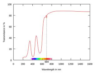
Due to the strong absorption lines in the blue and green range of the spectrum excited energy levels of the  $Cr^{3+}$  ion are populated by means of a flash tube. The  $Cr^{3+}$  ion can relax without electromagnetic radiation into a lower energy level, which corresponds to the small absorption line at 694 nm. Due to the small transition probability of this level, population inversion is achieved. Stimulated emission results in a pulse of laser light.
