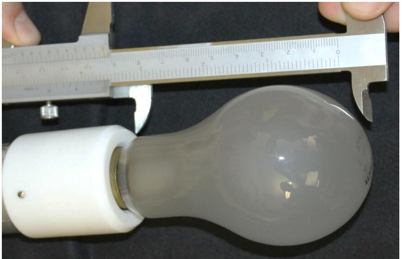
Figure 5 Incandescent light bulb RADIUM 100 W. Left top: installed in the goniometer. Right top: Measurement of the light bulb's diameter. Bottom: Measurement of the light bulb's height.
