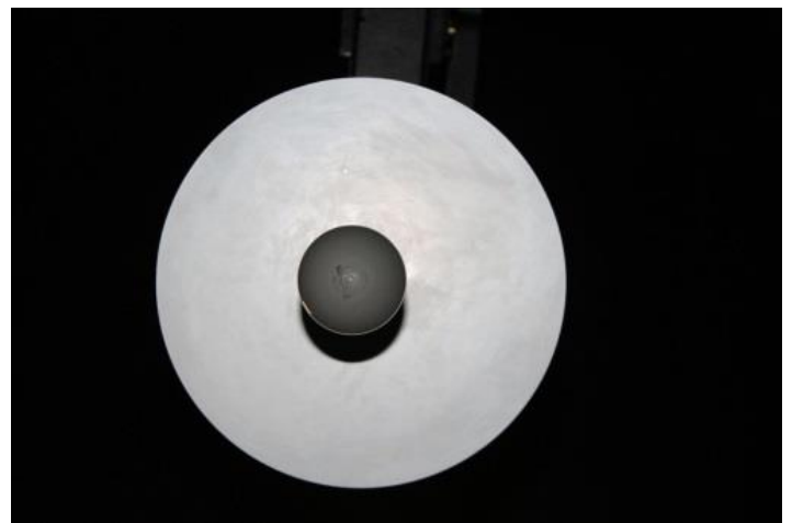
Figure 6 Reflector luminaire with matt plate. Left: installed in the goniometer. Right: bottom view.
