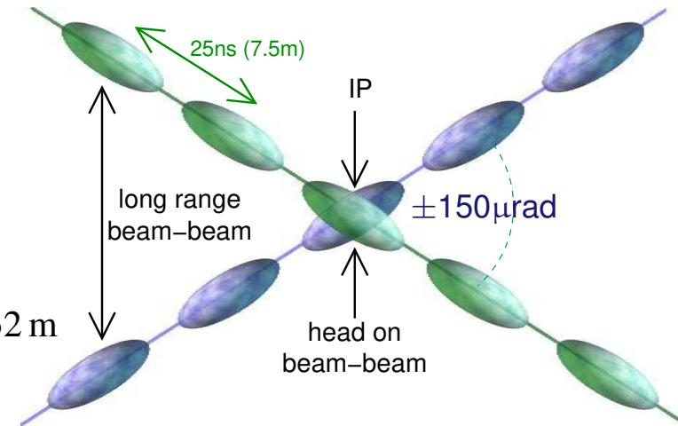
■ **Head-on:** Additional collisions for bunch separation below 232 m
