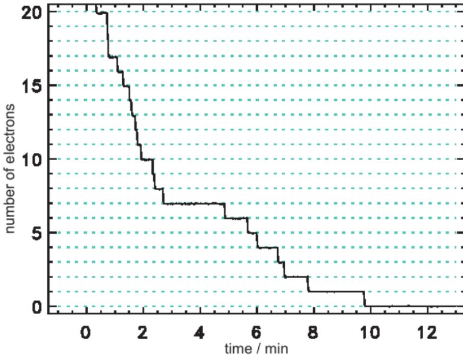
■ Counting individual electrons by measuring the decay of the synchrotron radiation intensity with cooled photodiodes
