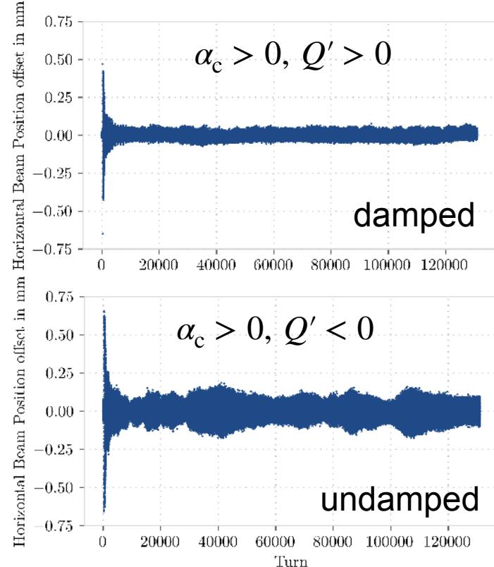
$$1/\tau_{\text{head-tail}} \propto \frac{U_0 \sigma_s Q'}{E_0 \alpha_c} I_b$$
